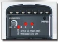
LED level meter for beam alignment.TWO LEDS on the receiver act as a level meter to visually disply the beam reception level. Each LED changes flickers more quickly→ flickers quickly→ flickers slowly→turns off. 7-level LED indicator enables quick and accurate beam alignment.
