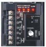
LED level meter for beam alignment. Three LEDS on the receiver act as a level meter to visually display the beam reception level. 10-level LED indicator enable quick and accurate beam alignment.
